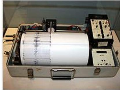
A seismograph made the graph below. The shaking recorded is due to an earthquake.
